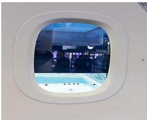
Figure 6 a. Electrochromic Virtual Window Blind On An Aircraft Cabin Window
